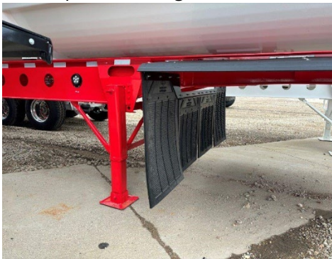
Mudflaps at Landing Gear
